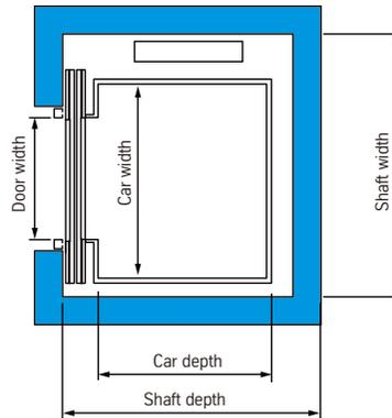
According to the elevator construction specification, the elevator shaft horizontal size is the minimum clearance by plumbing, and the allowed deviation as follows:
